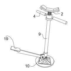
2. Attach (11) pillar base to (10) stand base. Check that both parts are secure to each other.
